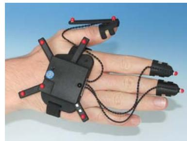
Figure 1: Finger tracking hardware.
